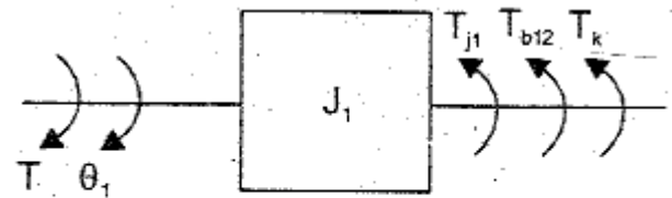
Fig 2 : Free body diagram of mass with moment of inertia J_1 .
