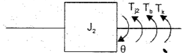
Fig 3 : Free body diagram of mass with moment of inertia J_2
